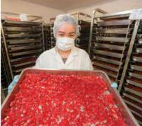
(Clockwise) A worker stirs one of five steam-jacketed kettles to prepare the liquid mass for depositing. After spraying a release agent on the moulds, 40 nozzles fill the cavities on their way to cooling. The starchless moulding line can produce pectin-base (pictured) as well as gelatin-based gummies. Depending on the formulation, curing ranges between 24 and 48 hours.
