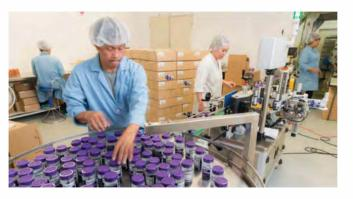
A WeighPack Systems complete solution automatically conveys, weighs and fills containers with its unique SpinDexer rotary indexing system designed specifically for vitamin gummies.
