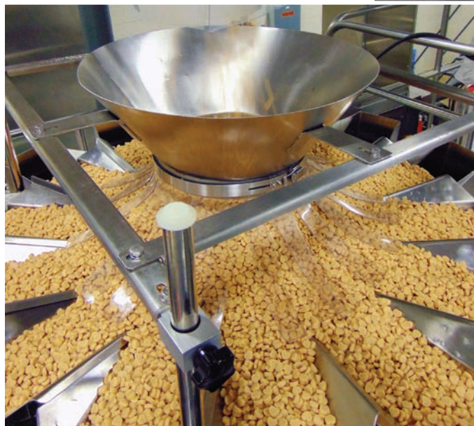
14 head CombiScale multi-head weigher accurately weighs and dispenses pet treats (left). Swifty Bagger 3600 automatically opens, fills, and seals pre-made pouches with zipper closures (above).
