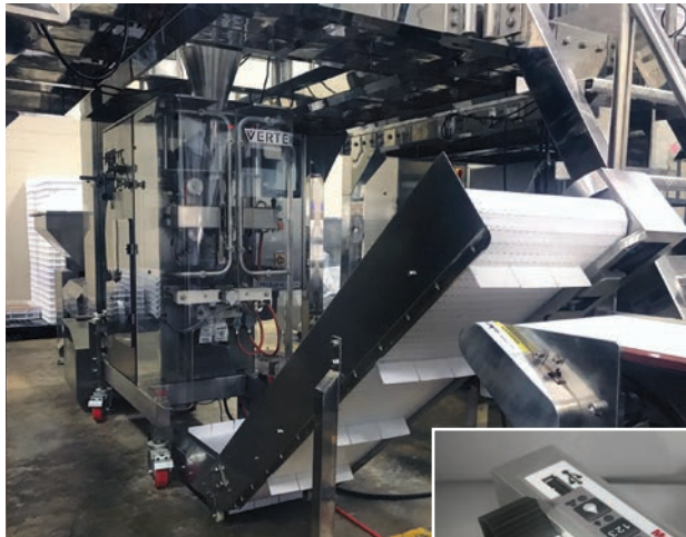
VerTek 800 vertical form & seal machine can produce pouches up to 8 inches wide and up to 60 packages per minute. Inset photo shows the cartridge-style digital thermal inkjet coding system that's integrated into the VerTek.
