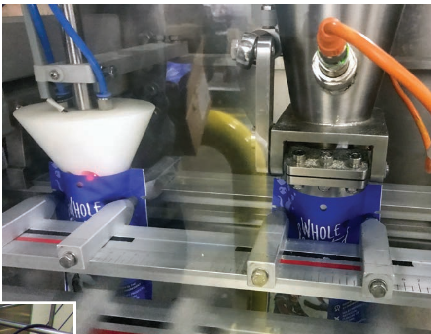
14 head CombiScale multi-head weigher accurately weighs and dispenses pet treats (left). Swifty Bagger 3600 automatically opens, fills, and seals pre-made pouches with zipper closures (above).
