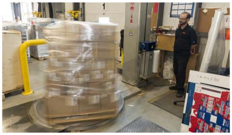
A finished mixed load of product is being secured to the shipping pallet by an automatic turntable stretchwrapping machine to ensure optimal product protection and load stability during transport.
