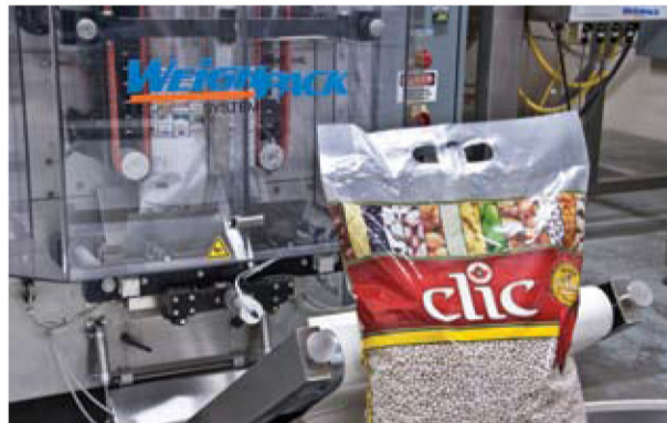
CLIC International is the first company to utilize its Vertek 1600 bagger to create plastic handles inline during the filling of 10-kilogram bags.
