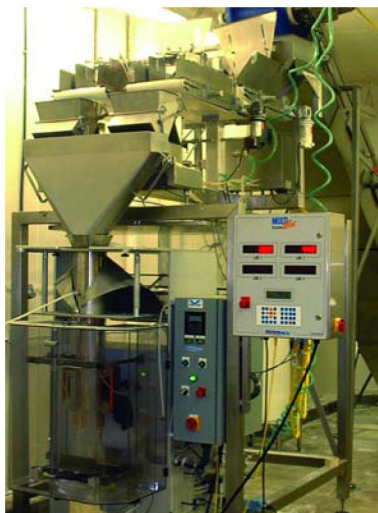
WeighPack Systems Twin Lane conveyORIZED Tiger Scale with VERTEK 1150 vertical form-seal bagger.
