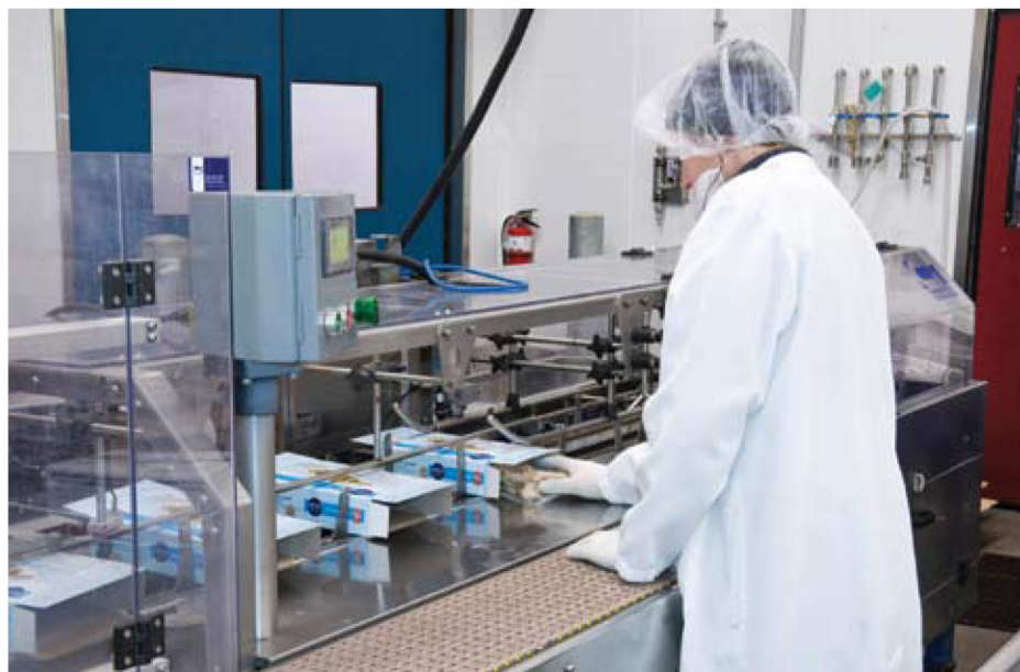
An operator places thermoformed packs of meat into a paperboard box erected by the HC 120 cartoner from Consolidated Technologies.
