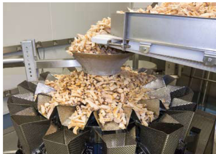
WeighPack's redesigned 14-head Primo Combination Multi-Head Weigher accurately dispenses chicken strips into the Xpdus Elite 1200 vertical bagger positioned underneath.
