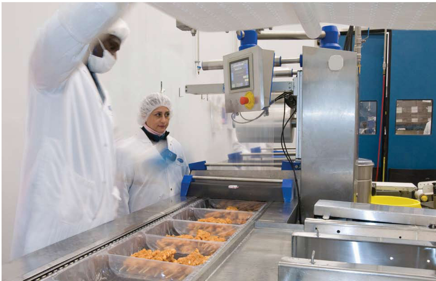
Machine operators monitoring one of two Repack RE20/5 thermoforming systems used by Expresco to package satays, strips and marinated meat skewers for both its raw and cooked product lines.
