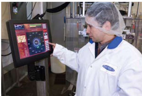
Maintenance technician Khalid Fazroun uses the operator-friendly color touchscreen HMI to program the WeighPack Xpdus Elite 1200.
