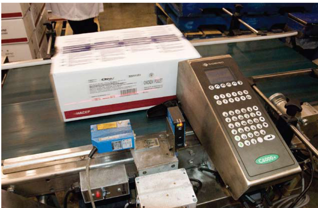
A master carton containing boxes of frozen seasoned chicken kebobs has lot code data applied to it by a Domino C6000+ inkjet printer.
