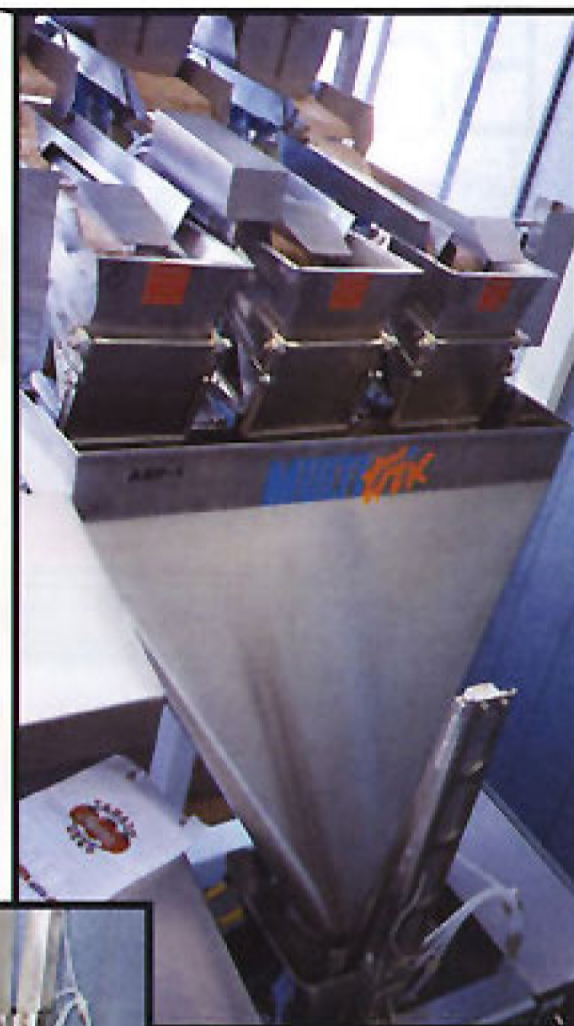
Weigh/fill/bagging system, top left, has an accuracy of +/- 1 gram (300 seeds). As the bag leaves the heating section, it passes a rotary cutter, left, that removes the plastic material above the seal. To start each fill cycle, an air jet blows downward to open the top of the bag, above, after which a plunger descends to completely open the bag plus "pop out" the bottom gusset.
