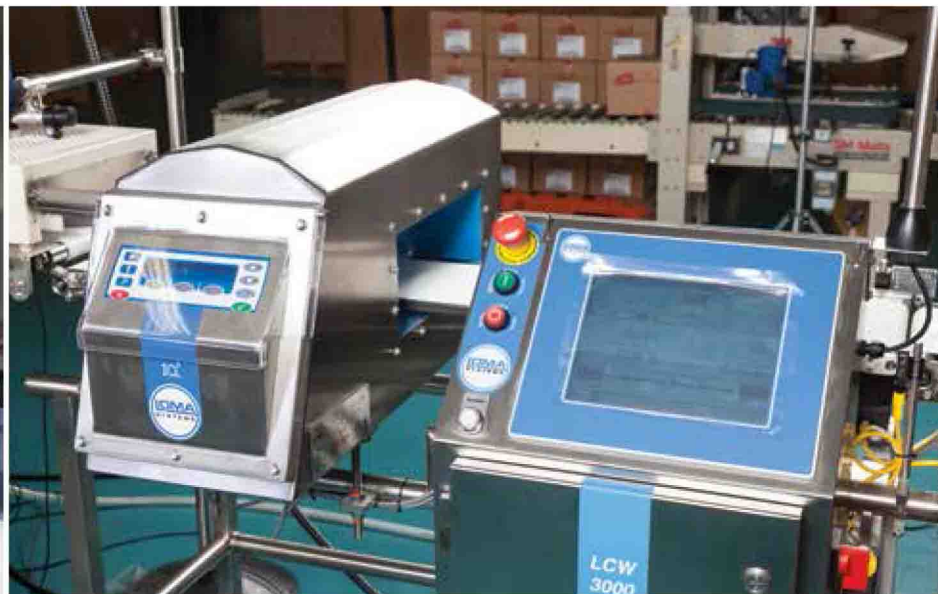
The Quebec City plant operates four Loma Systems metal detection units and one LCW 3000 checkweigher system to ensure optimal product quality and weight accuracy.
