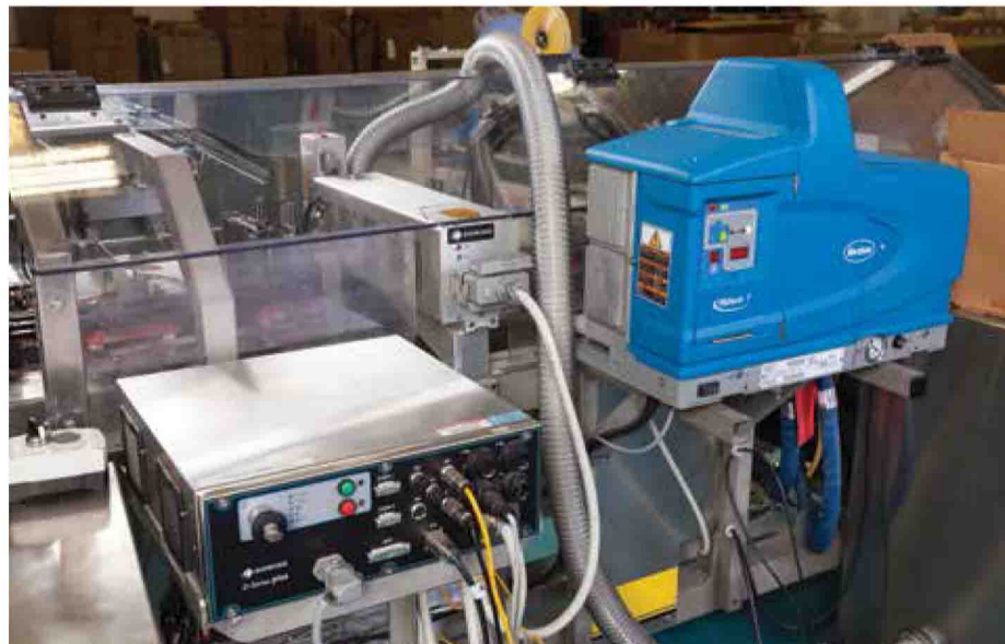
The reverse side of a D100+ laser coder, inscribing lot-code data onto a paperboard package before it is sealed by Nordson's ProBlue 7 hotmelt adhesive applicator.
