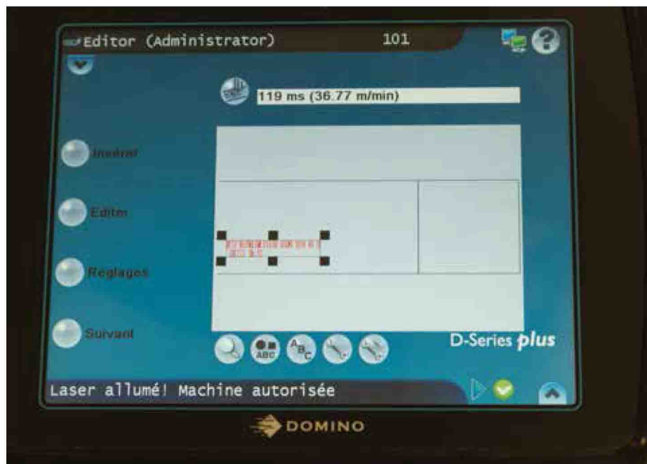
A close-up of the easy-to-use control panel on the D100+ laser scribing system used to mark the outer packaging, either tray boxes or bar wrappers, with the best-before data.
