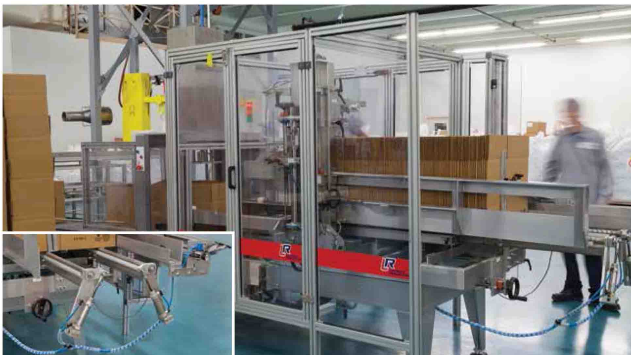
A Leclerc Robotique case-erector uses Festo pneumatics ( inset ) to form corrugated cartons in a swift, gentle motion.
