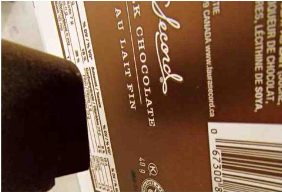
A close-up view of the Domino D100+ laser coder quickly applying best-before data and lot-code information onto the Laura Secord 40-gram Milk Chocolate bar wrapper.
