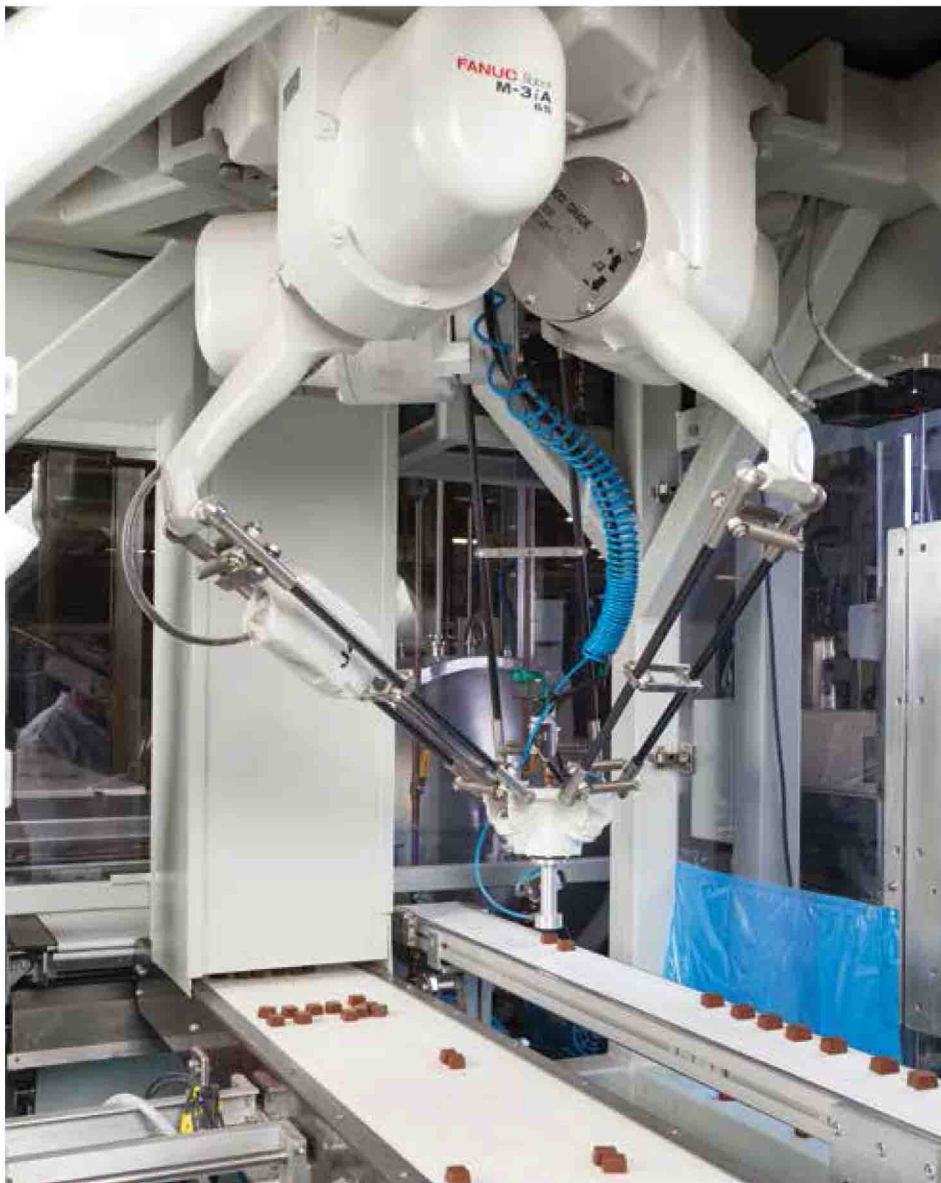
A Leclerc Robotique machine uses a Fanuc Robotics M-3iA/6S robot for quick and accurate pick-and-place of individual chocolate pieces from one line onto another.
