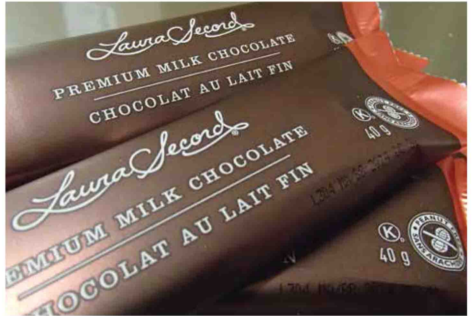
The finished product of a 40-gram Mik Chocolate bears a permanent laser-scribed coding applied by the Domino D100+ coder at the Laura Secord/Nutriart plant.
