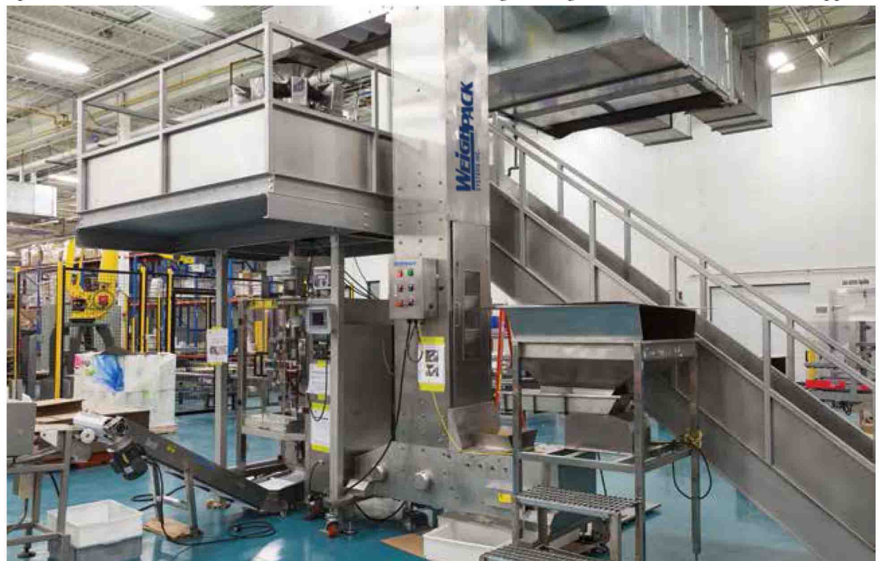
Laura Secord / Nutriart utilizes a 10 Head PrimoCombi 2.5L multihead weigher and XPdius vertical form & seal bagging machine, manufactured by WeighPack Systems to ensure accurate pack fills of chocolates produced at the company's 250,000 square-foot facility in Quebec City.
