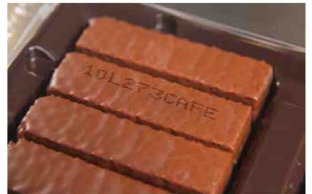
A close-up view of clean, legible lot code data applied to the thin protective layer of film covering chocolate-coated cookies by a Domino A320i inkjet printer.
