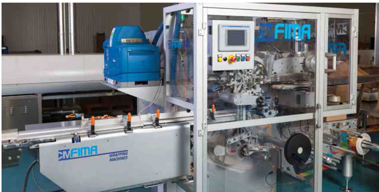
Featuring a Rockwell Automation Allen-Bradley PanelView Plus 700 operator touchscreen, the easy-to-use CM Fima wrapping machine, manufactured by Carle & Montanari, quickly foil-wraps individual pieces of chocolate.
