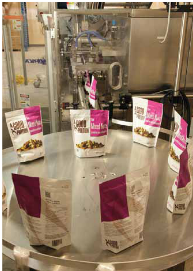
A Swifty Bagger SB-3600 machine from WeighPack Systems incorporates a user-friendly Allen-Bradley PanelView Plus 600 touchscreen interface to facilitate high-accuracy filling of flexible stand-up pouches at up to 45 pouches per minute.
