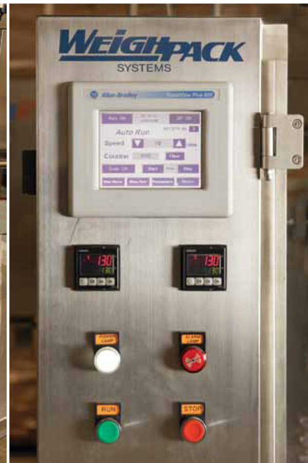
A Swifty Bagger SB-3600 machine from WeighPack Systems incorporates a user-friendly Allen-Bradley PanelView Plus 600 touchscreen interface to facilitate high-accuracy filling of flexible stand-up pouches at up to 45 pouches per minute.
