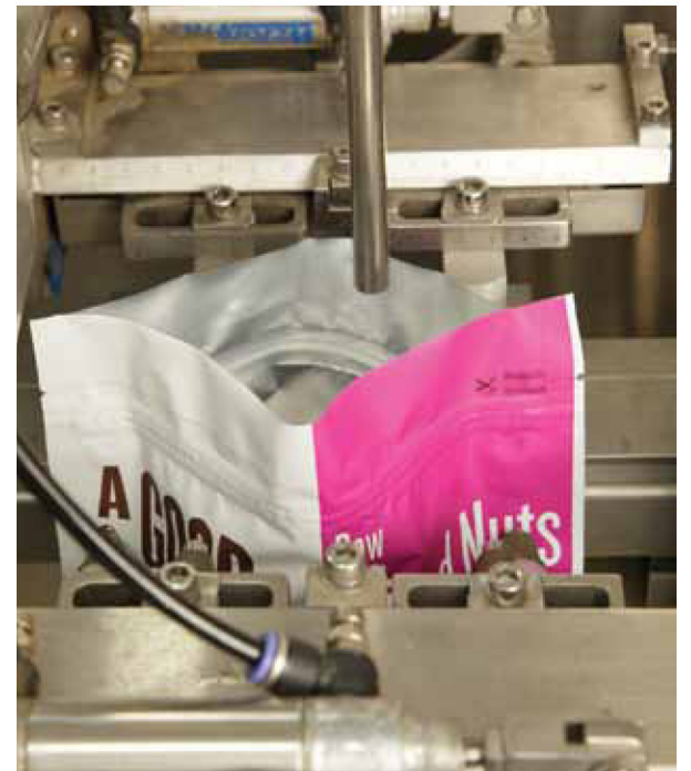
A close-up view of the 454-gram and 907-gram zippered stand-up pouches used for NaturaPack's A Good Portion brand of beans, pulses and nuts packaged and sealed on the Swifty Bagger SB-3600 machine manufactured by WeighPack Systems.
